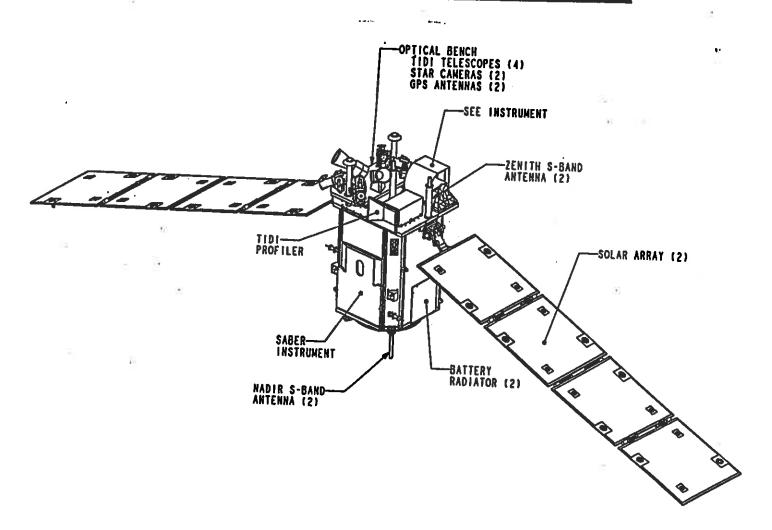
For a satellite in a low orbit, the path loss to a ground station is a strong function of the angle from nadir. If the satellite is stabilized in an earth-oriented direction, the radiation pattern of the antennas can be shaped to favor the larger angles from the -Z axis. This results in some improvement to the worst-case communication links.
