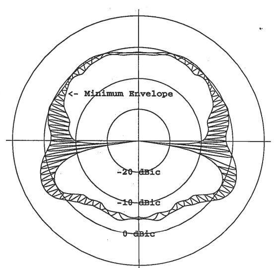
The effects of the spacecraft structure on the performance of the antennas will be determined both by testing on a full-scale mock-up of the satellite body (minus the large solar panels) and by numerical modelling. The numerical work will use Version 3 of Ohio State's Numerical Electromagnetic Code - Basic Scattering Code (NEC - BSC) which was originally developed for similar NASA Space Station studies.
