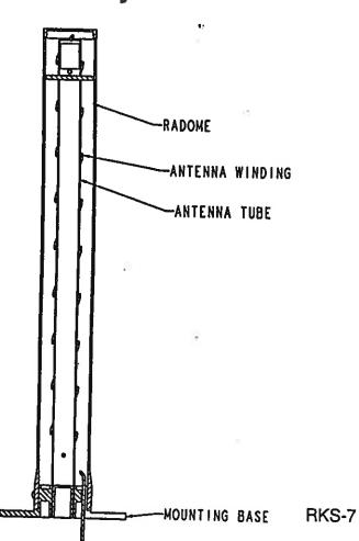
The type of antenna being used for the zenith directed hemispherical coverage application is a resonant quadrifilar helix. Variations of the basic design have been flown on numerous APL spacecraft. Shown in the photograph are two examples which flew on the Charge Composition Explorer Satellite.
