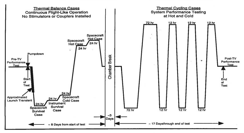
Tests will be performed during spacecraft thermal vacuum to include:
