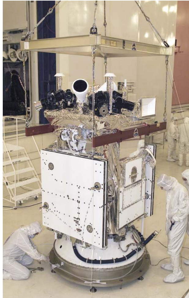
Figure 4. TIMED assembled to the flight payload adapter. The spacecraft in the launch configuration awaits integration into the dual payload adapter fitting launch vehicle system. The lifting fixture is still attached.
