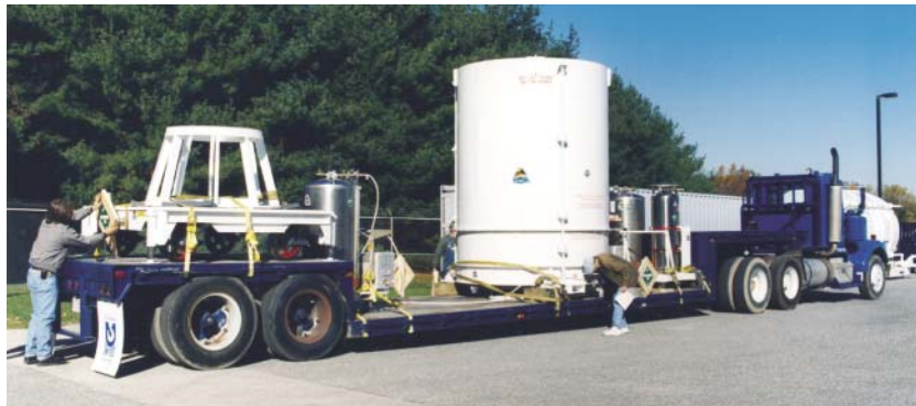
Figure 1. TIMED spacecraft shipment. The spacecraft (inside the container) is secured for land shipment to Andrews Air Force Base.
