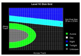
The Level 1C data products contain data directly measured by the sensors, such as photometer counts, uncertainties, light intensities and pointing information derived from the GUVI raw sensor data and the TIMED Satellite ephemeris data. The data are gridded into a GUVI based coordinate system consisting of the along orbit position of the sensor and the angle of the scan from the nadir position. This gridding eliminates overlap from scan to scan due to the large instantaneous
