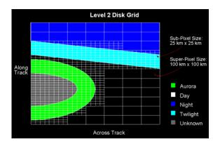
The Level 2B data products contain environmental parameters which are derived from the sensor data by scientific algorithms specific to day, night, and auroral regions. The data is averaged into 100 x 100 km² resolution to form "super pixels" on the day and night and 25 x 25 km² for the auroral products. The "super pixels" are then processed by the algorithms to yield geophysical parameters which are calculated from the radiance of the different colors.
