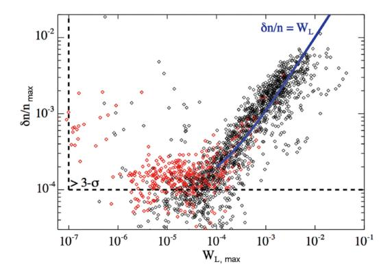
**Figure:** Maximum observed density fluctuations  $\delta n/nmax$  vs. the maximum electric energy of electron plasma waves WL,max, in the electron foreshock (black diamonds) and the free solar wind (red diamonds). The blue line represents the expected level of density fluctuations generated by Langmuir nonlinear ponderomotive effects. The black dotted lines show the 3-sigma detection levels. More than three years of STEREO/WAVES data are summarized in this plot.
