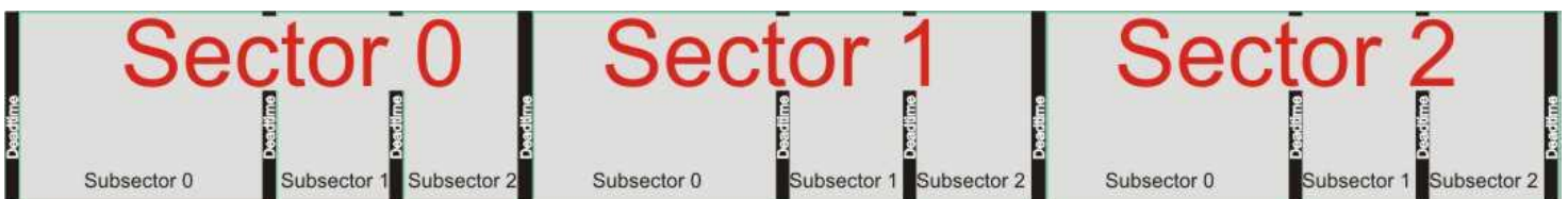
Figure 3-1 Sector and subsector scheme used by RBSPICE also showing inter-subsector dead times.
