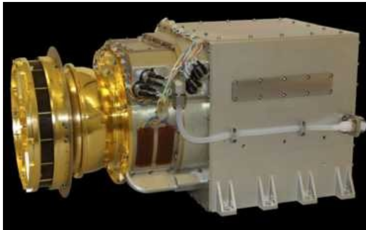
Figure 5-1 Completed HPCA Flight Model 1
