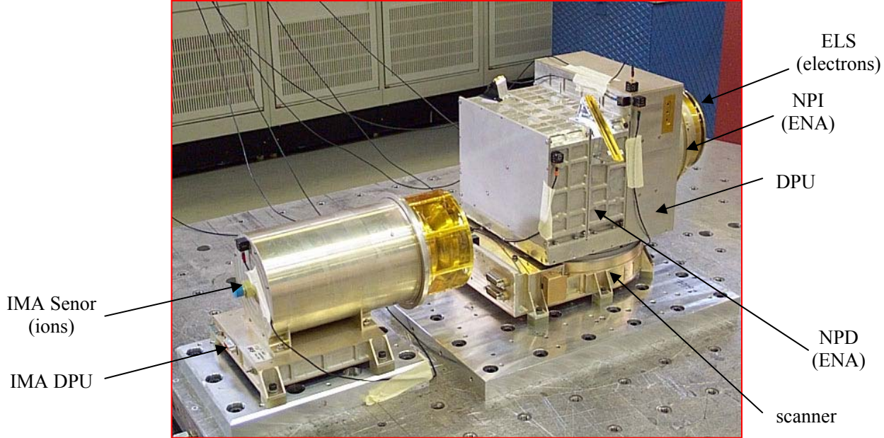
Figure 6. Shown here is the ASPERA-3 experiment undergoing vibration testing. The main unit (right) is mounted on the top of the Mars Express spacecraft and contains the ELS, NPI, and NPD instruments mounted on a scanner. The IMA unit (left) is mounted on the bottom of the spacecraft. The ASPERA-4 experiment on Venus Express spacecraft uses mostly modified Flight Spare units from Mars Express instrumentation and will be flown in the same configuration.
