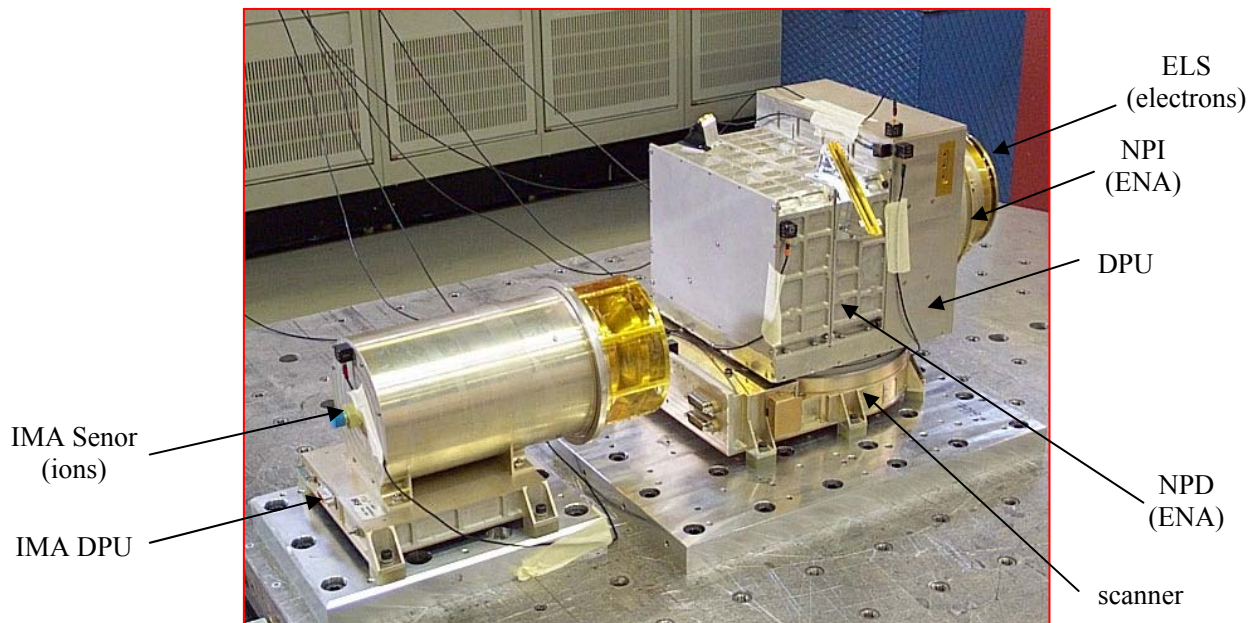
Figure 7. Shown here is the ASPERA-3 experiment undergoing vibration testing. The main unit (right) is mounted on the top of the Mars Express spacecraft and contains the ELS, NPI, and NPD instruments mounted on a scanner. The IMA unit (left) is mounted on the bottom of the spacecraft. The ASPERA-4 experiment on Venus Express spacecraft uses mostly modified Flight Spare units from Mars Express instrumentation and will be flown in the same configuration.
