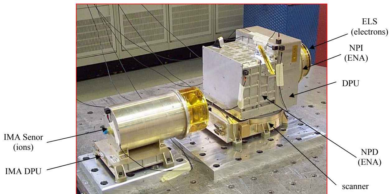
Figure 2. Shown here is the ASPERA-3 experiment undergoing vibration testing. The main unit (right) is mounted on the top of the Mars Express spacecraft and contains the ELS, NPI, and NPD instruments mounted on a scanner. The IMA unit (left) is mounted on the bottom of the spacecraft. The ASPERA-4 experiment on Venus Express spacecraft uses mostly modified Flight Spare units from Mars Express instrumentation and will be flown in the same configuration.
