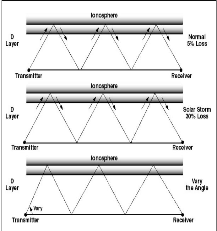
Calculate the remaining signal strength for each bounce from the transmitter to the receiver. Determine the amount remaining at the receiver's location. Round the answers to the nearest whole number.
