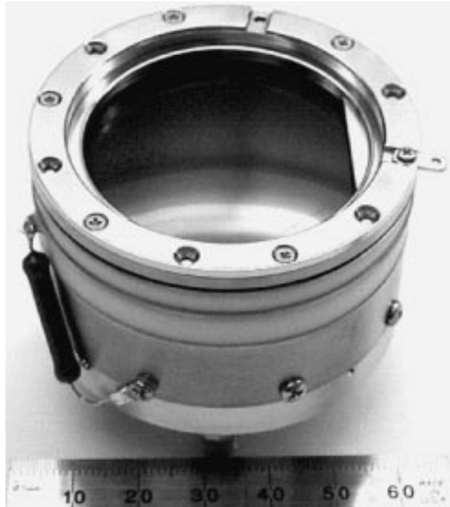
Figure 13. Photograph of the EUV curved surface flight MCP sensor. The active area is 4 cm in diameter, and its radius of curvature is 7 cm.
