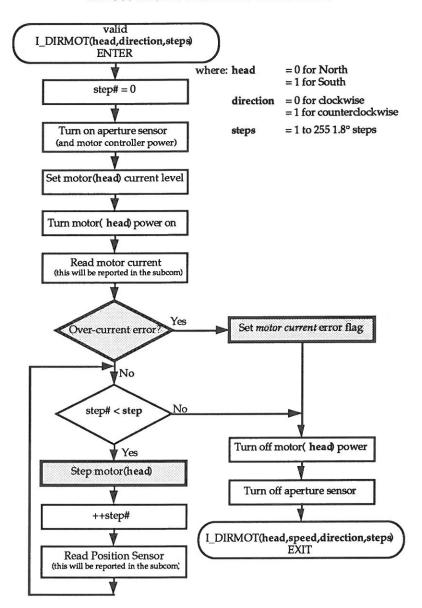
This flowchart moves the wheel only 1.8 degrees per step. The phototransistors are checked only to provide this information in the subcom housekeeping.
