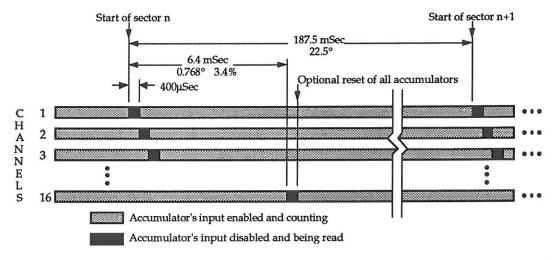
The desired method for STICS is option A and for ICS is option B,. Note that in both cases an accumulator is always reset to zero after it is read.
