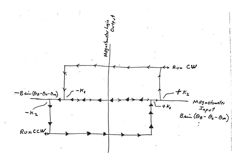
Figure 3. Alternate Double Hysteresis Loop Control Logic
