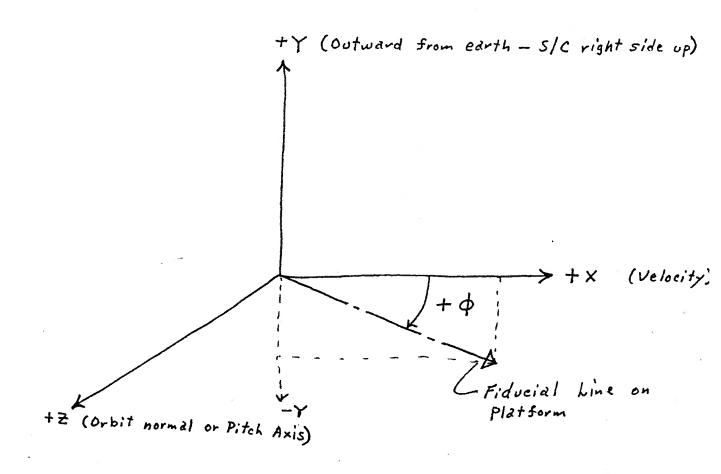
Figure 1. Coordinate System and  $\boldsymbol{\varphi}$  Definition
