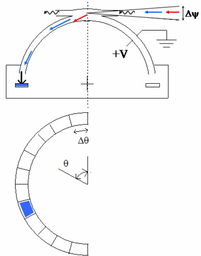
The detector is a half-annular microchannel plate, MCP (to amplify the signal corresponding to an incident electron). The charge from the MCP is collected on an anode, which can detect which of twelve  $15^\circ$  sectors the electron arrived in. Signals are collected during 4 millisecond intervals. The electric field in the analyser is varied through a range of energies, to cover the full energy range several times per spin.
