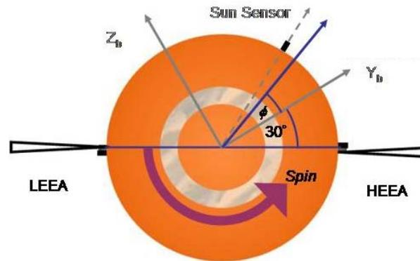
The PEACE instruments are designed to use the pair of sensors to characterise  $f(v)$  the velocity distribution function of electrons in the plasma environment local to the spacecraft for an energy range from the spacecraft potential up to 26 keV.
