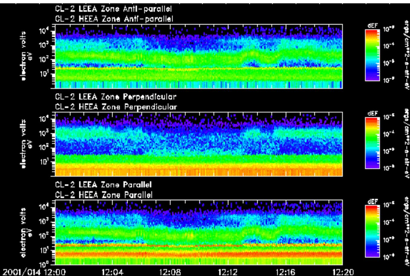
Note that the two segments are collected half a spin apart. Each is a snapshot: a single energy sweep
