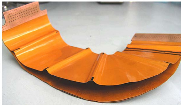
After First Layer Bends Complete
