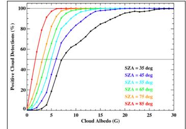
**Figure 3**. Estimated CIPS cloud detection sensitivity. Each curve corresponds to CIPS measurements at a fixed solar zenith angle (SZA), from 35  $^{\circ}$  to 85 $^{\circ}$ . For a given cloud albedo (x-axis, in units of  $1G=10^{-6}\,\mathrm{sr^{-1}}$ ) the curve shows the probability of detection (in %). For example, a 5 G cloud will be detected 50% of the time at 55 $^{\circ}$  SZA and 97% of the time at 85 $^{\circ}$  SZA.
