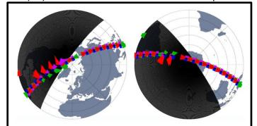
**Figure 3.** Example of CIPS sampling for full-orbit Continuous Imaging including eclipses. Pole-centered views are shown for the NH (left) and SH (right); black shading indicates the night side. For illustration only; the exact geometry varies from orbit-to-orbit and day-to-day.
